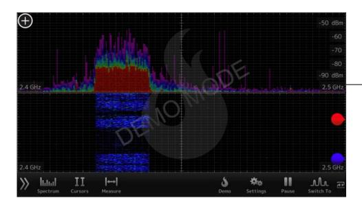
The screen is split into two views. The top view is **Real Wave**. This represents real time spectral data.
