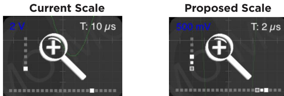
The blue number in the top left corner shows your volts per division and the white number in the top right corner shows the timescale. Focus on the right image. The two solid dots show where you're headed and the white outlined dot shows your current scale.
