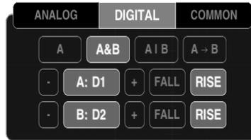
Then, the option that is touched will activate. From the menu, select the desired triggering function from these options: single channel only **A**, simultaneous events on two channels **A&B**, a single event on one of two channels **A|B**, or concurrent events on two channels **A->B**.
