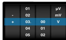
To select the desired trigger level touch and drag in each of the four columns until the specific value is reached. To activate the settings touch away from the menu. When analog triggering has been enabled, then all the advanced options for digital triggering will be grayed out.
