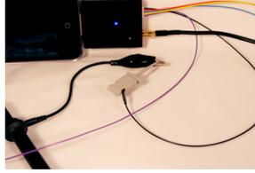
Remove the connector attachment from the analog probe. Then connect the SMD grabber for D1 (or the purple wire) to the tip of the analog probe.
