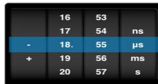
To select the desired trigger delay touch and drag in each of the four columns until the specific value is reached. To activate the settings tap away from the menu or tap **BACK**.
