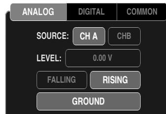
To navigate to an exact trigger level touch on
