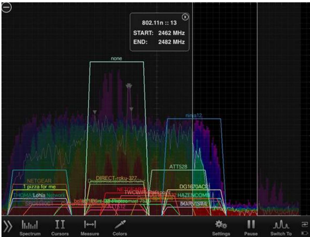
? In this example, there is no clear channel in 2.4 GHz. This interference was limited to the inside of the home (interference was not visible when leaving the residence). In this example although 2.4 GHz was very congested, 5 GHz was not. It was recommended that the customer add dual band adapters on wireless devices to utilize 5 GHz for best speeds...or accept slower speeds on 2.4 GHz.
